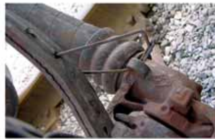
View of a deformed glad hand clip
